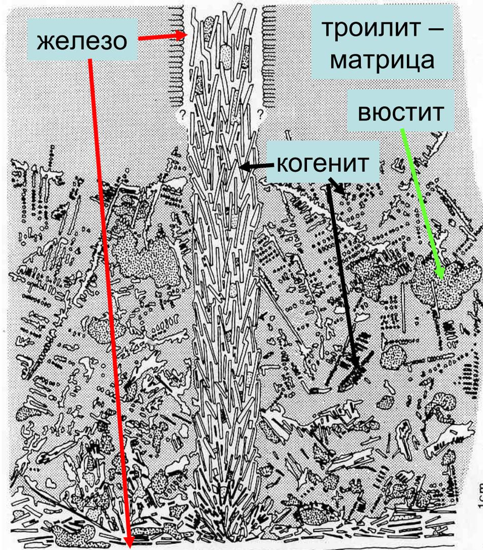
FIG. 5. Vertical section through the dendrite zone (DZ) and the lower part of a columnar iron-cohenite eutectic dendrite of iron-coated cohenite laths with interstitial troilite and wüstite. The iron mantle and cellular iron-troilite intergrowth formed early during solidification of TZ. Sketch composed from several sections. White laths: cohenite; white: iron; light dotting: troilite; dense dotting: wüstite pseudomorphs.
