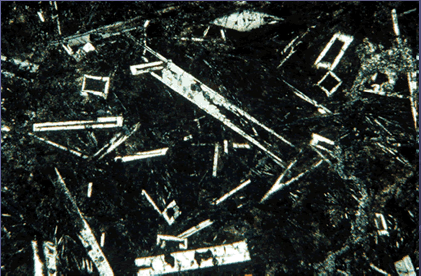
Basalt from Hole 856H, Middle Valley, Juan de Fuca Ridge, Leg 169. Field of view = 2.5 mm, cross-polarized light. Plagioclase phenocrysts in basaltic glass show hopper-car, boxy, and acicular habits.
