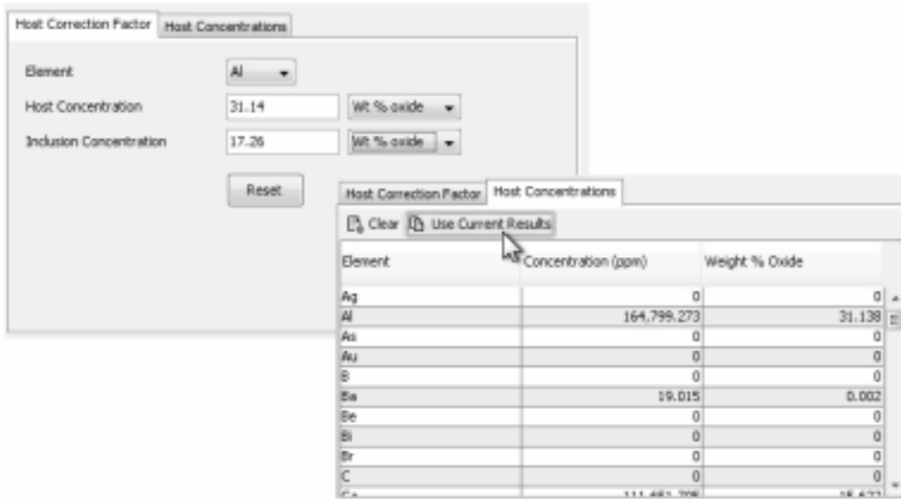
FIG. A5-9. Host correction window in AMS to enter the concentration of the element that will be used to deconvolve the mixed signal from the host and MI.
